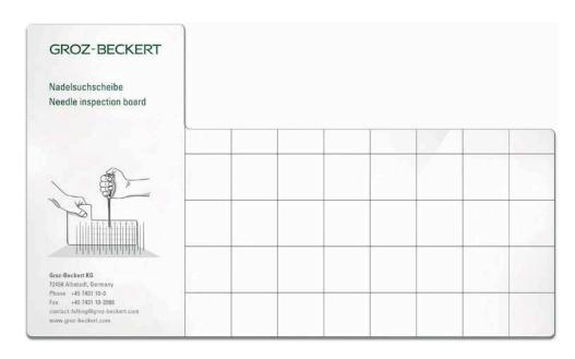
In order to locate broken needles among the large number of needles in the board, the needle inspection board from Groz-Beckert is guided row-by-row through the needles, by the user crosswise to the machine direction. Every needle can thus be checked and broken or damaged needles located and replaced if necessary. Equipped needle boards can also be checked using the needle inspection board to ensure that all needles are aligned correctly. This check can be
