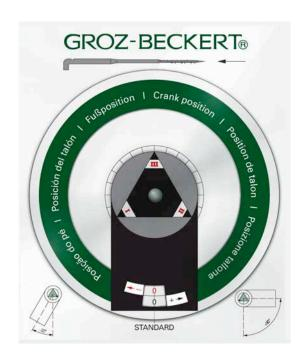
When it comes to crank positioning, Groz-Beckert refers to the needle perspective looking at the needle point with the crank aligned downwards. With the aid of this disk, all possible scenarios can be depicted and clearly indicated for users. This allows users to simulate the relative rotary position between the crank and working part while looking at the needle crank/at the rear of the disk, and to then take a reading of the number of degrees at the front of the disk
